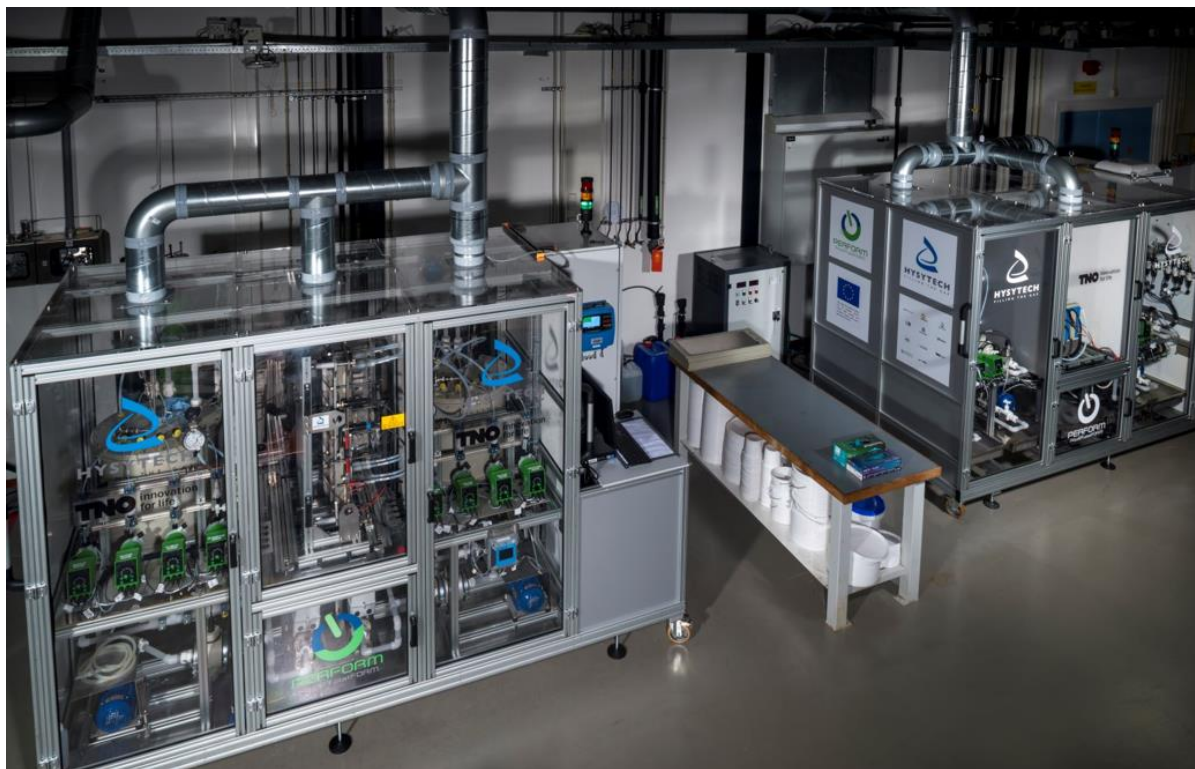
Picture - Pilot equipment in the TNO laboratories, designed by the partners in the PERFORM project and constructed by HYSYTECH. On the left the UPS electrochemical pilot with a 1m 2 surface area reactor. On the right: Electro dialysis unit.
